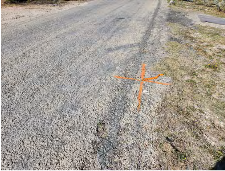
Figure 6. Ground control point established for aerial photogrammetry.
