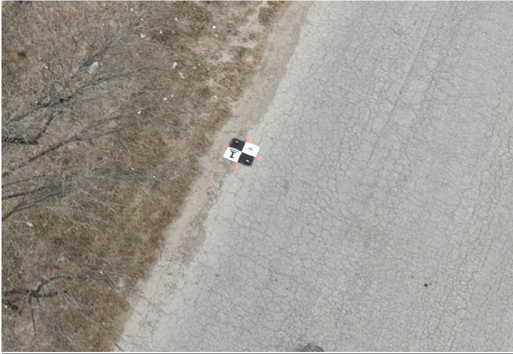
Figure 7. Ground control point established for aerial photogrammetry.
