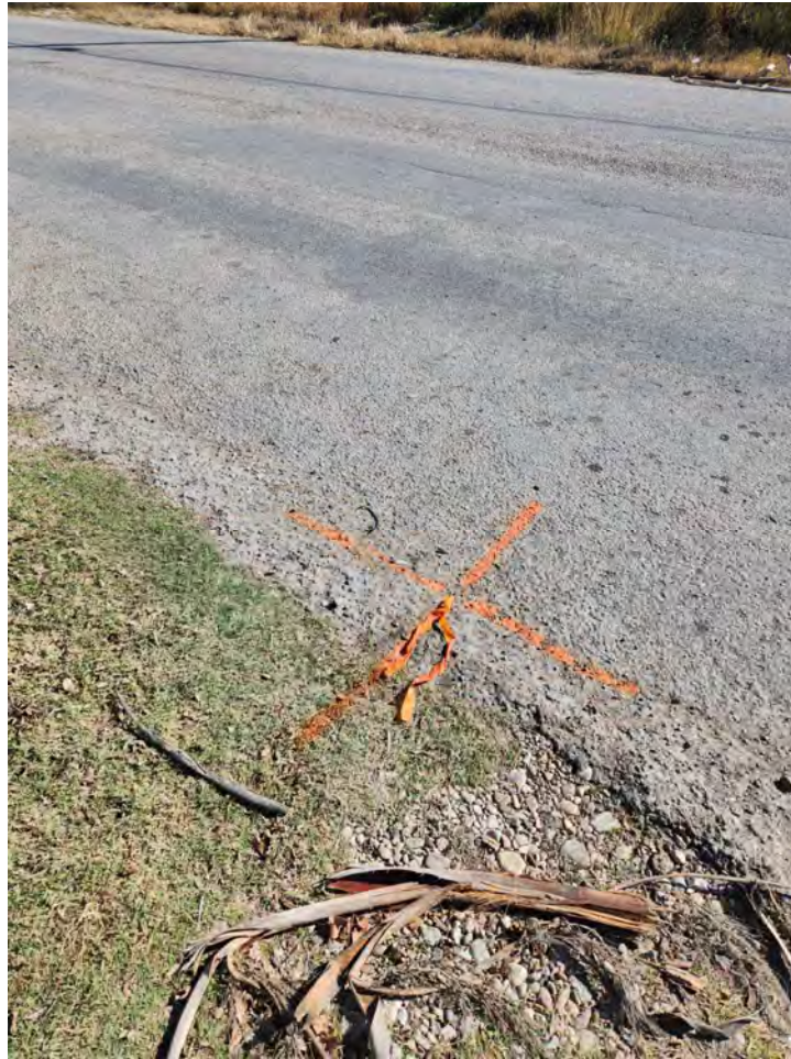
Figure 7. Ground control point established for aerial photogrammetry.
