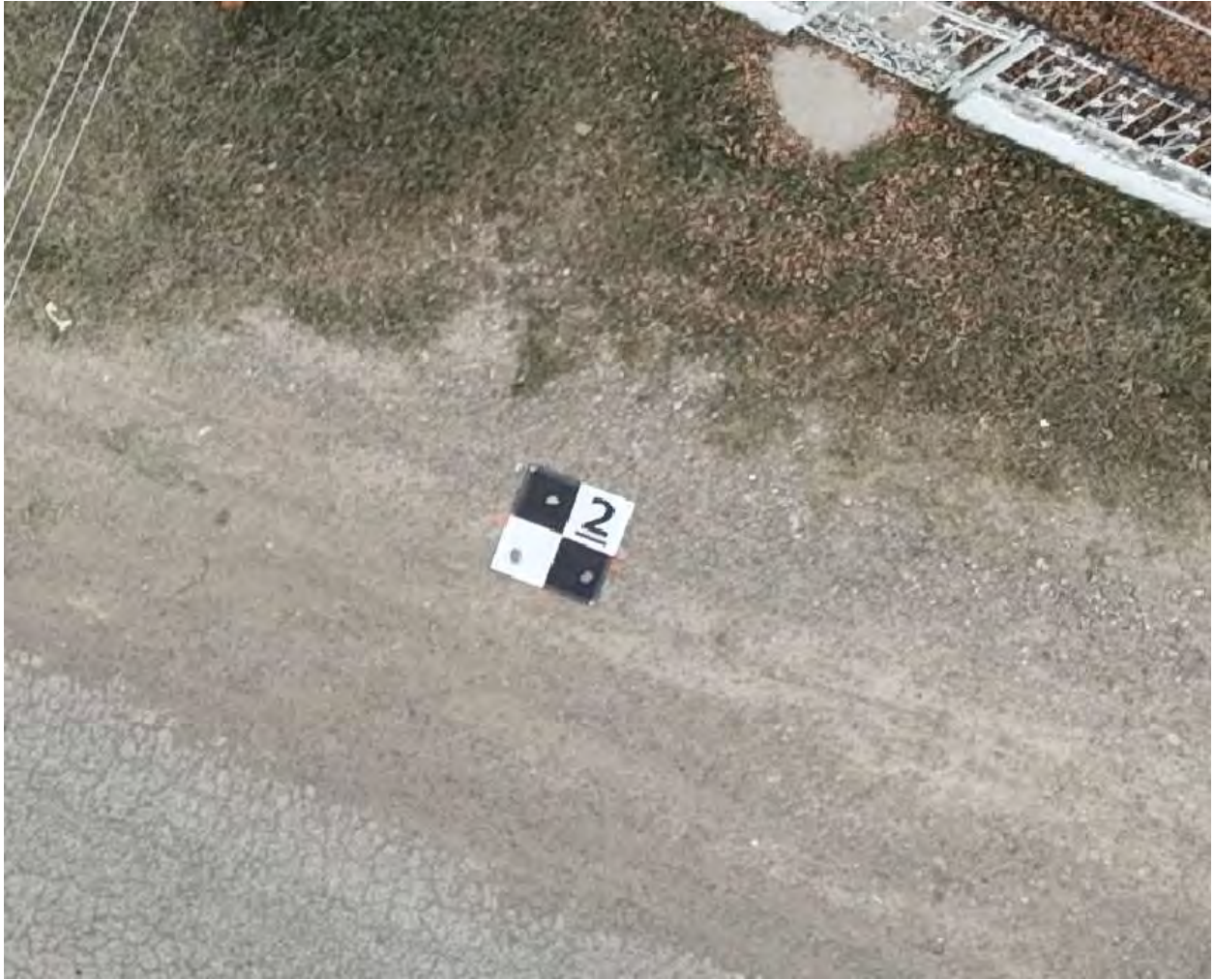
Figure 6. Ground control point established for aerial photogrammetry.
