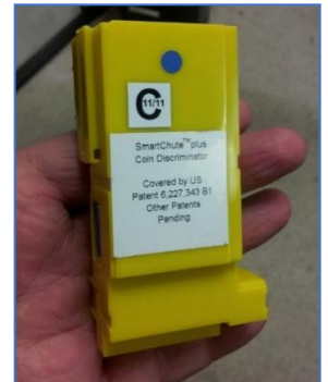
Figure 7 - MacKay's SmartChute coin acceptor
