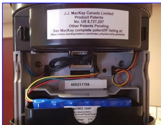
Figure 4 - Rechargeable lithium ion battery pack (blue) shown inside the mkORA
