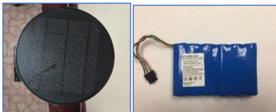
Figure 5 - rechargeable lithium-ion battery pack and large solar panel on the top of the mkORA
