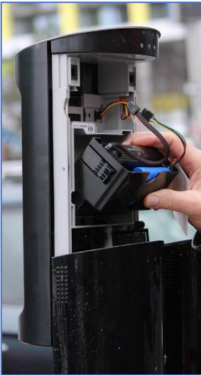
Figure 2 - mkORA opened for maintenance
